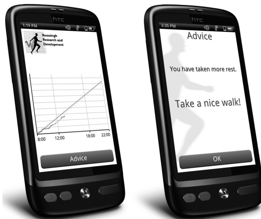
Figure 5.1: Screenshots of the activity coaching application. On the left: cumulative physical activity plotted over a reference activity line indicating the user's goal between 08:00 and 22:00. On the right: example of an encouraging motivational cue.
