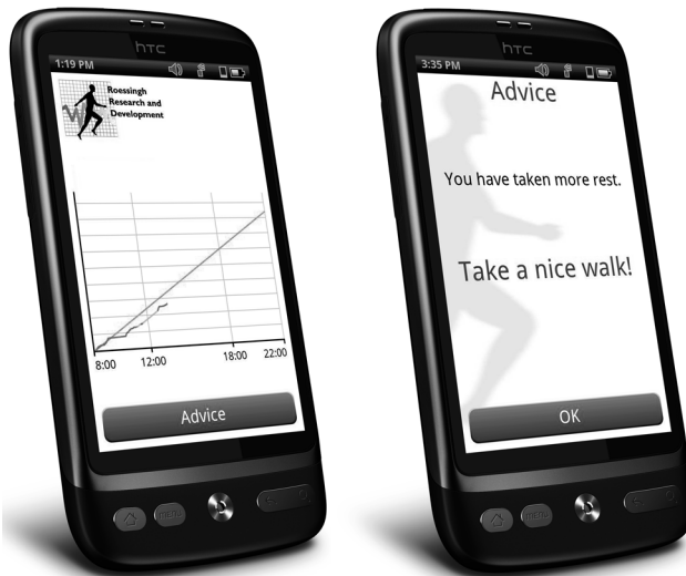
Figure 3.1: Screenshots of the activity coaching application. On the left: cumulative physical activity plotted over a reference activity line indicating the user's goal between 08:00 and 22:00. On the right: example of an encouraging motivational cue.
